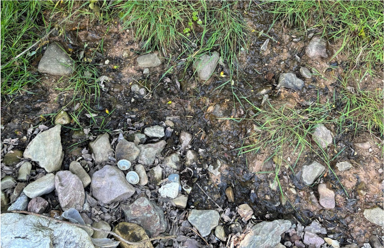
Figure 8 View of the seepage at the cliff toe mid-way between cross-sections E and F
