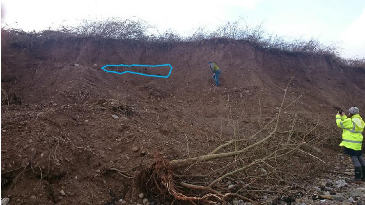
Figure 10 Sand lens in the slope failure
