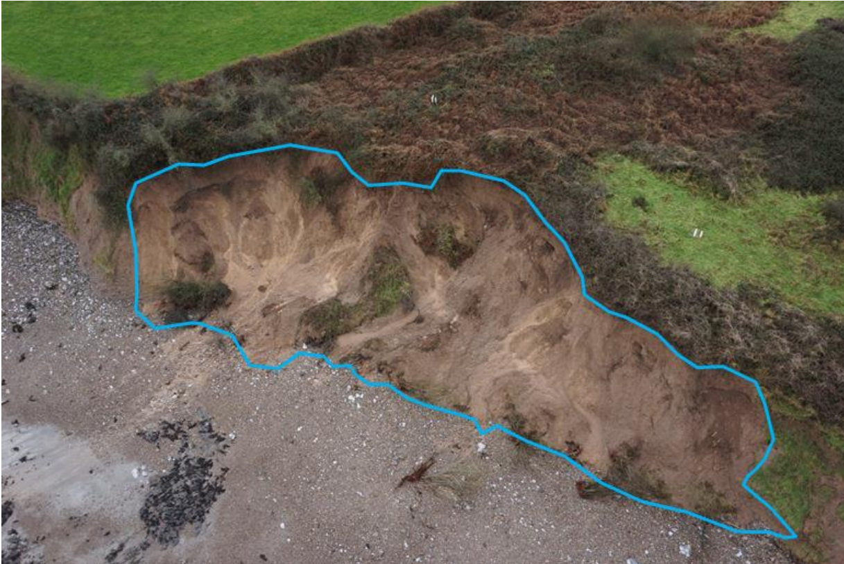
Figure 3 Drone photography showing slope failure to the southern section
