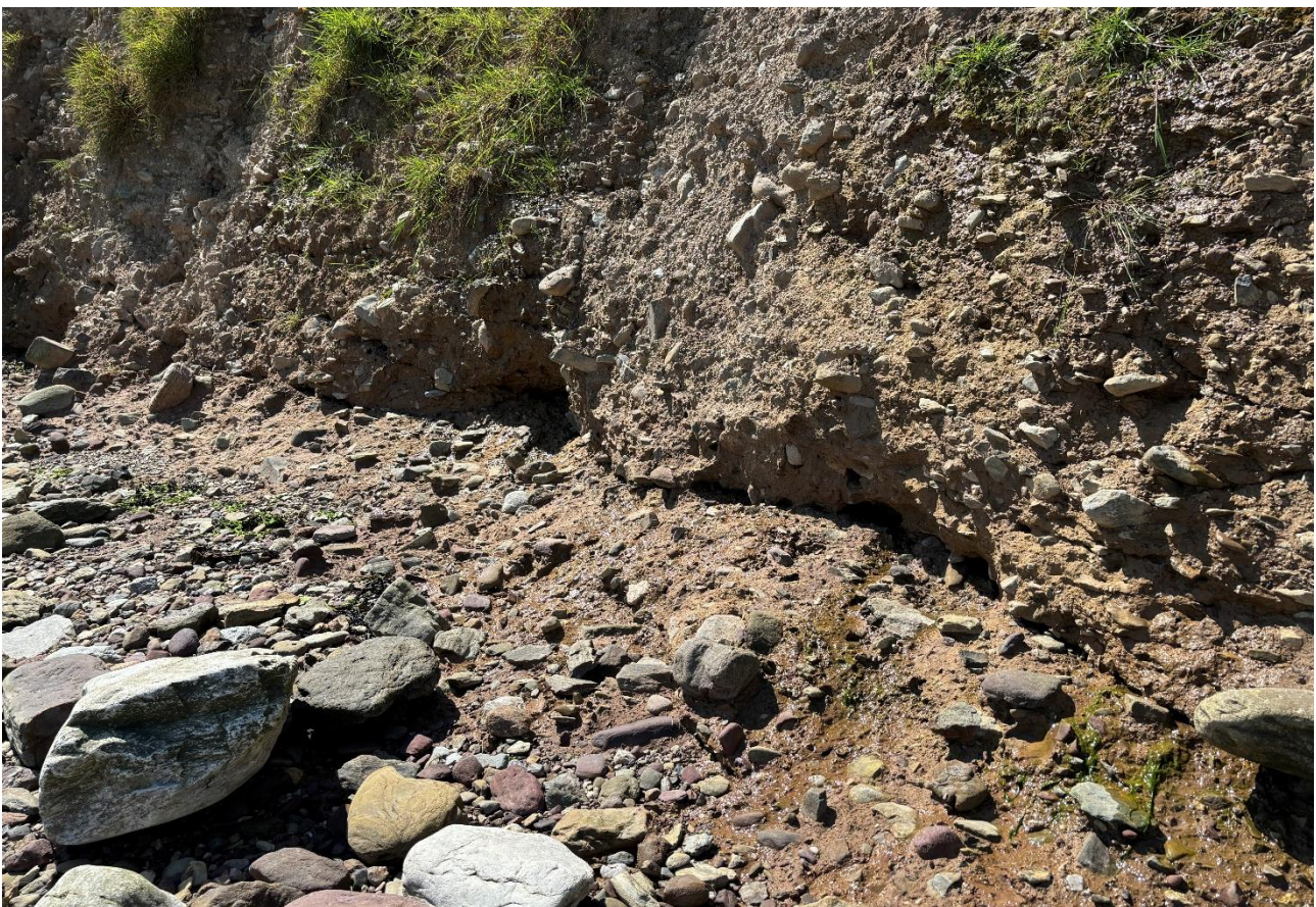
Figure 24 View of cliff toe notching and seepage at the southern site boundary limit
