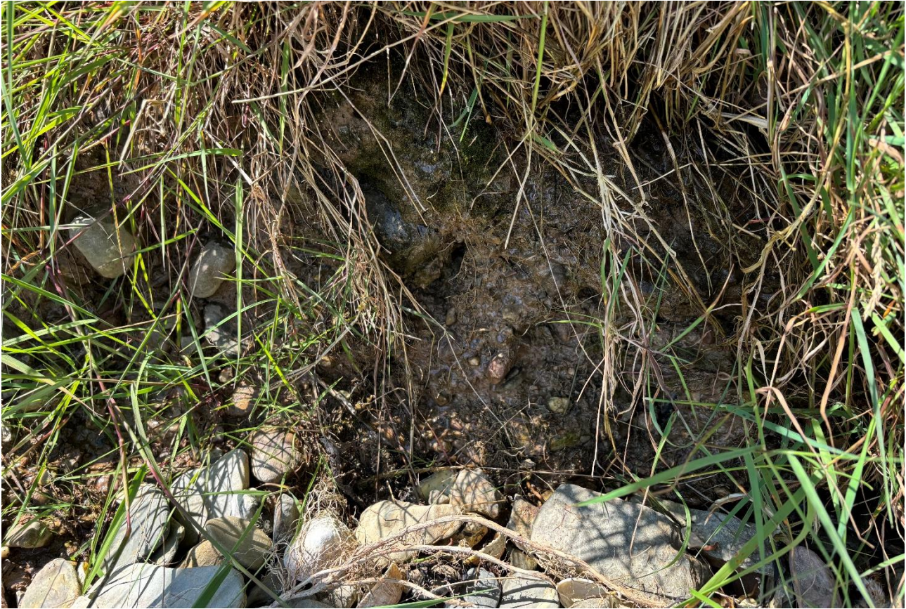
Figure 25 View of seepage at the cliff toe between cross-sections F and G
